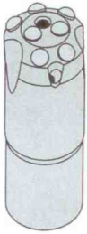
Model -17 2+3 gauge buttons, 2 front buttons. One front and two side flushing holes.
