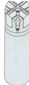
Cross-type bit 4 chisel inserts in cross formation. Traditional insert bit for extremely abrasive rock formations. Ideal for soft formations that cause "snake-skin" problems for carbide. Produces straight holes but has lower penetration than button bits.
