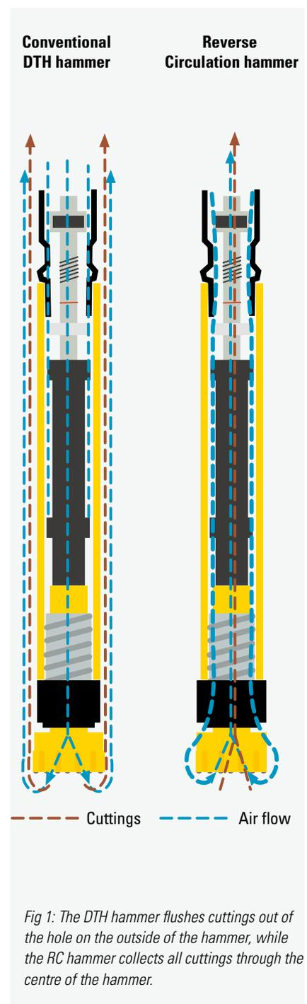
Fig 1: The DTH hammer flushes cuttingts out of the hole on the outside of the hammer, while the RC hammer collects all cuttingts through the centre of the hammer.
