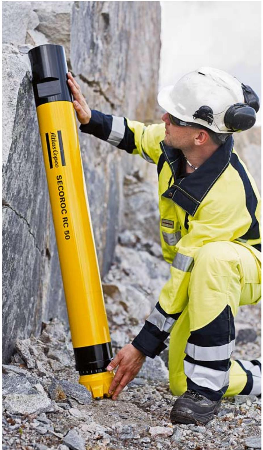
The RC50 hammer from Atlas Copco Secoroc is designed for both deep hole exploration drilling and In-Pit grade control.
